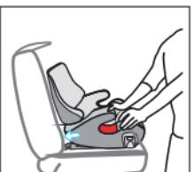
Push two locking arms firmly into the insert guides until heard an audible sound "click" on both side. If the ISOFIX is locked favorably and correctly, a green mark will turn up on the release button, please do check it.
