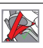
Pull the vehicle seat belt across and secure it in the normal way. The lap belt shall be routed under both the armrests of the child seat and the diagonal belt shall be routed above the armrest of the child seat.
