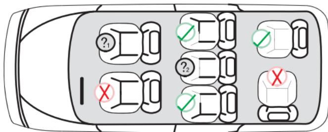
① Not to be used on this seat if a Passenger front airbag is active.
