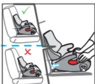
Grasp the seat body to check the seat if it is fastened tightly or shakes, If the seat shakes and the locking arms are pulled out, please repeat the above steps and install it again.
