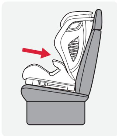
Push the child car seat in the direction of car seat back, ensuring there is no space between the child car seat and car back.
