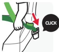
Put the child seat in the vehicle, and put your child sitting on the child seat. Put the upper part of vehicle safety belt through the hooker in the headrest, the lower part of vehicle safety belt through the armrest, then lock the safety belt buckle. Then tighten up the vehicle safety belt.
